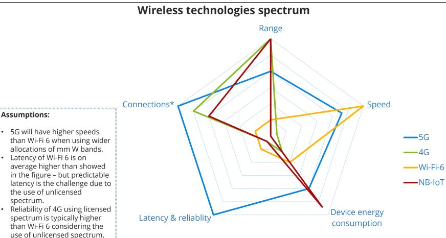
Although 5G does not yet provide optimal results for all these dimensions simultaneously because of current technological and infrastructure limitations, it will eventually become the technology of choice for critical communications that require extreme reliability and service quality, including those within industrial settings. However, not all performance dimensions can be maximized at the same time. There are trade-offs between speed, range, energy efficiency, and latency.
